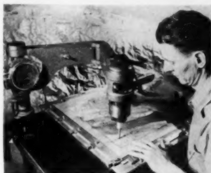
The thin-gauge aluminum sheet is formed and shaped into the master model with the Reliefograph. The operator works from the reverse side of the model—and high points are pushed down, rather than thrust up.
